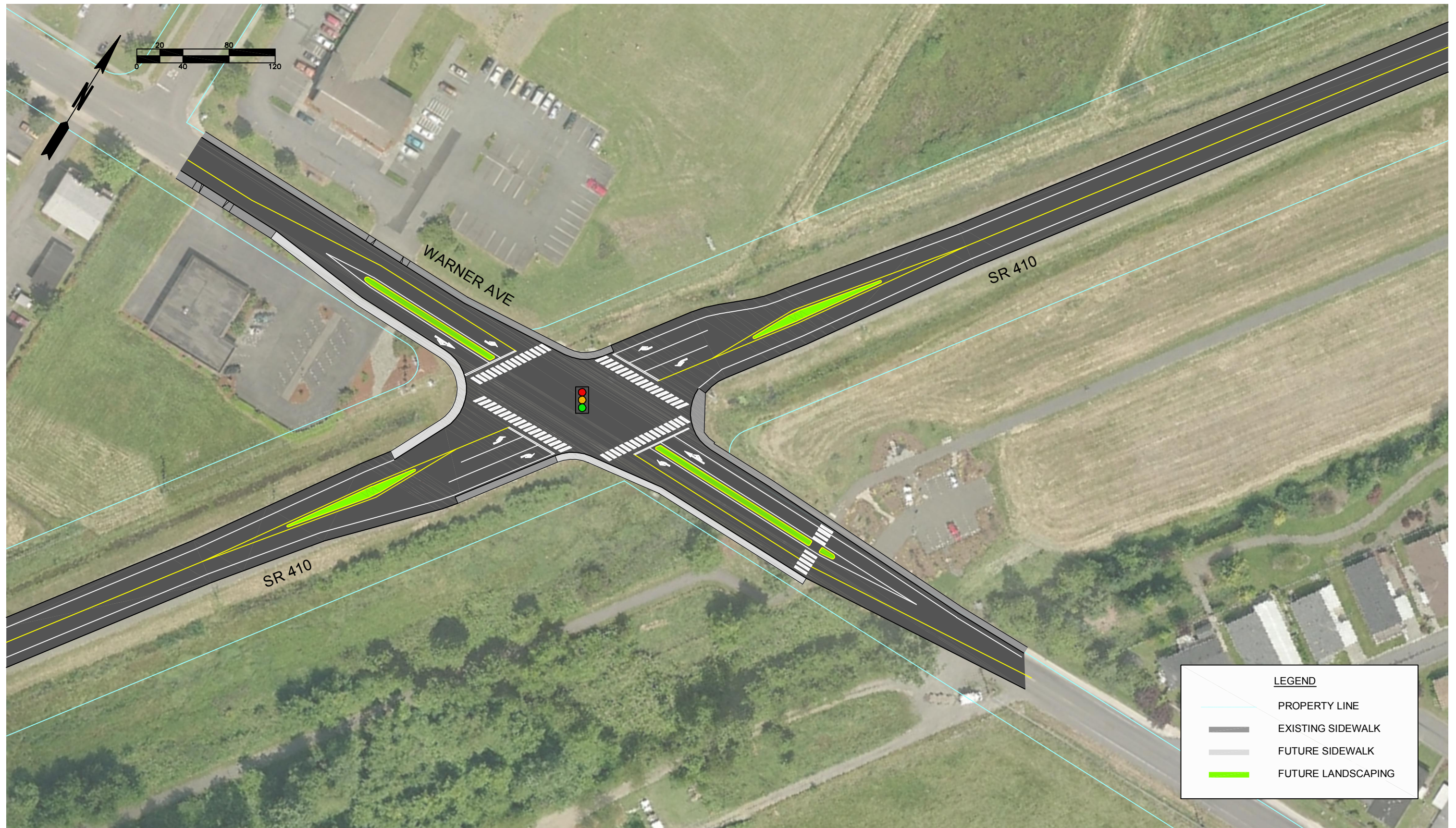
Segment 1: Warner Avenue Intersection - Widen Out Approaches
