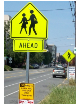
Multiple approach signs may be used to indicate pedestrian crossing activity, particularly for unsignalized intersections
